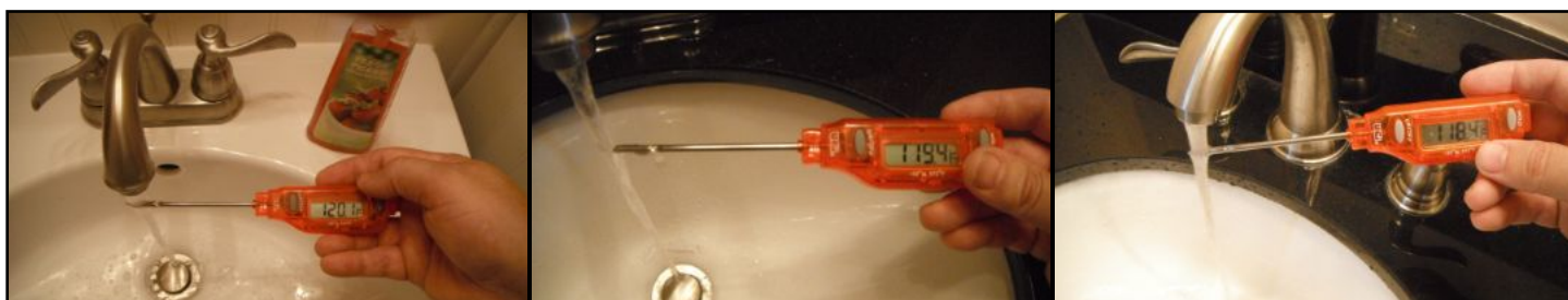
120 degrees hot water main floor 119.4 degree hot water upstairs 118.4 degree hot water upstairs
